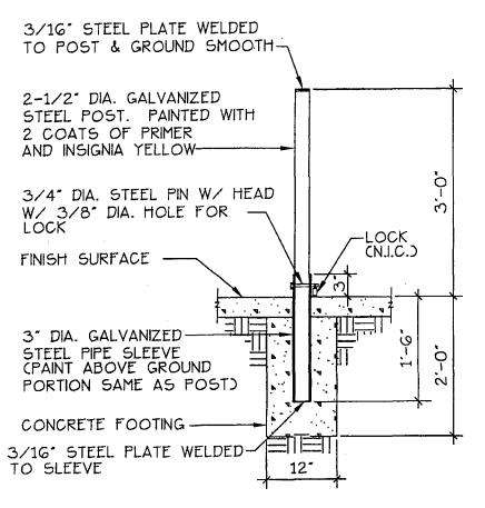
NOTE: DRILL A 13/16" DIA. HOLE THRU BOTH THE POST AND SLEEVE FOR PIN PLACEMENT.
