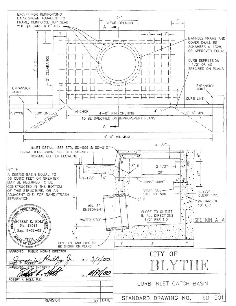
WHEN THE BASIN IS TO BE CONSTRUCTED WITHIN THE LIMITS OF A PROPOSED SIDEWALK OR IS CONTIGUOUS TO SUCH A SIDEWALK CONCRETE SHALL BE CLASS "3" CONCRETE WHICH SHALL ATTAIN A 28—DAY COMPRESSIVE STRENGTH OF 4000 PSI IN ACCORDANCE WITH ASTM C39/C39M—99. THE TOP OF THE BASIN SHALL BE POURED MONOLITHIC WITH SIDEWALK, USING CLASS "3" CONCRETE IN THE SIDEWALK. THE TOP OF THE CATCH BASIN SHALL BE FINISHED PER SIDEWALK STANDARDS.
