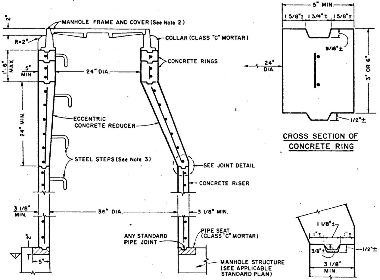
**VERTICAL SECTION OF MANHOLE SHAFT**
