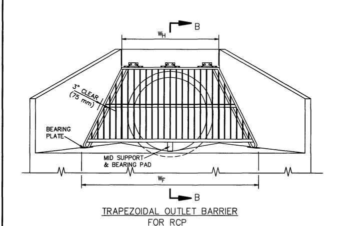
FOR TRAPEZOIDAL OUTLET BARRIERS, USE  $W_{\mbox{\scriptsize H}}$  TO DETERMINE NUMBER AND SIZE OF HINGES AND USE  $W_{\mbox{\scriptsize F}}$  TO DETERMINE REQUIRED FRAME MEMBER SIZES.
