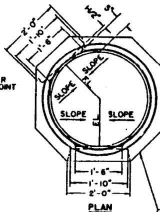
INVERT SECTION DIMENSIONS TYPICAL AS CASE 1 EXCEPT AS DETAILED HEREON
