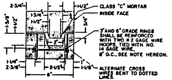
NOTE: REINFORCEMENT STEEL SHOWN SHALL APPLY TO GRADE RINGS ONLY.
