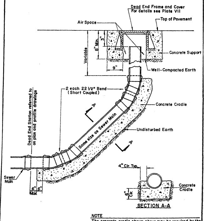
The concrete cradle shown above may be required by the City Engineer when a firm and unyielding foundation is not obtainable.
