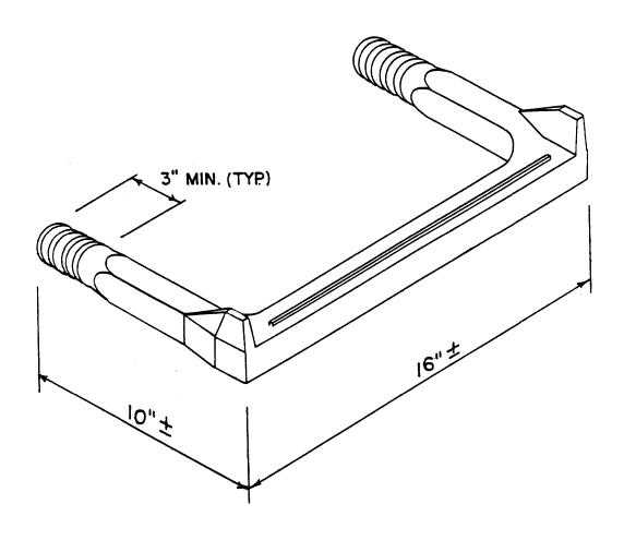
THE MANHOLE STEP SHALL BE INJECTION MOLDED COPOLYMER POLYPROPYLENE WITH A CENTER CORE OF 1/2" STEEL REINFORCEMENT. THE STEP SHALL COMPLY WITH ASTM C-478.
