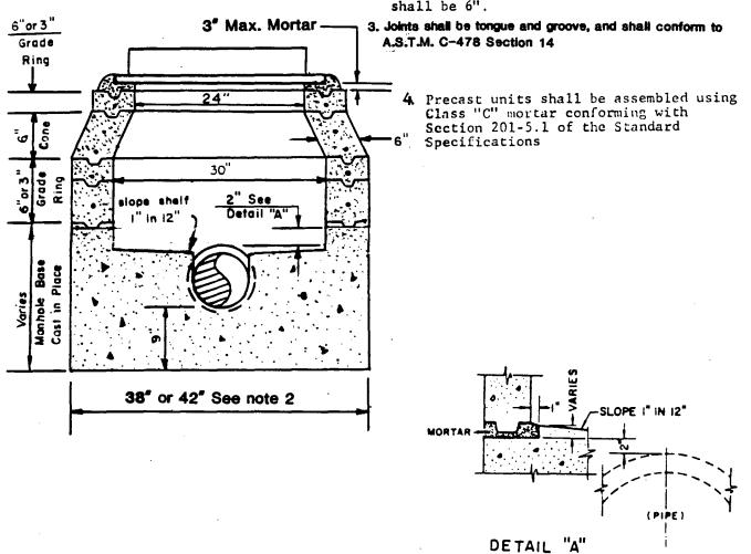
THE FOLLOWING STANDARD PLANS ARE INCORPORATED HEREIN: 616 MANHOLE FRAME AND COVER
