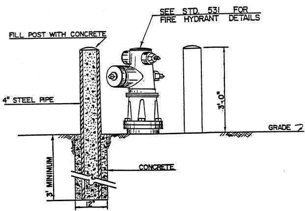
THE FIRE HYDRANT GUARD POST SHALL RECEIVE ONE PRIMER COATING OF NO. 5210 YELLOW CHROMATE PRIMER FOLLOWED BY ONE COAT OF NO. 5176 CORROSION INHIBITIVE RED PRIMER AS MANUFACTURED BY GILMORE NOLAN OR APPROVED EQUAL. FINISH PAINT SHALL BE TWO COATS RUSTLESS INDUSTRIAL NO. 2420 FIRE HYDRANT CHROME YELLOW PAINT OR APPROVED EQUAL.
